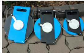
Optic-acoustic water level meters G 10 – G 30
