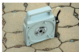
Oil-film gage measuring instrument / OWI 10 - OWI 30
